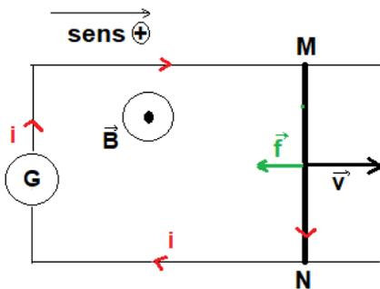
$$i = \frac{-1}{R} \frac{d\Phi}{dt} \quad \text{avec} \quad \Phi = \vec{B} \cdot \vec{S} = B \cdot S = B \ell vt$$
