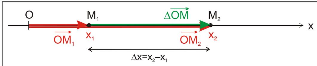
$$v_{mx} = \frac{(\Delta\vec{OM})_x}{\Delta t} = \frac{(\vec{OM}_2)_x - (\vec{OM}_1)_x}{t_2 - t_1} = \frac{x_2 - x_1}{t_2 - t_1} = \frac{\Delta x}{\Delta t}$$
