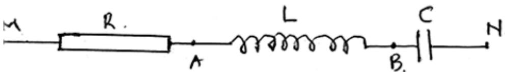
$$\left. \begin{array}{l} L\omega = 314 \\ \frac{1}{c\omega} = 159,23 \end{array} \right\} L\omega > \frac{1}{c\omega}$$
