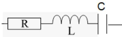
$$\omega_0 = \sqrt{\frac{1}{LC}} \quad \text{AN : } \omega_0 = 100 \text{ rad/s}$$
