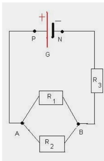
$$R_1 = 10\Omega; R_2 = 5\Omega; R_3 = 5\Omega$$
