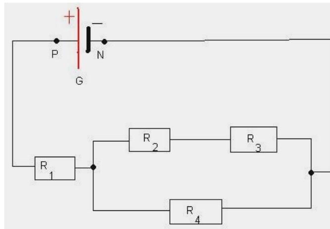
$$R_1 = 2 \Omega; R_2 = R_3 = 4 \Omega; R_4 = 16 \Omega$$
