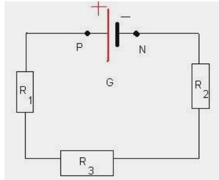
$$R_1 = 60\Omega; R_2 = 20\Omega; R_3 = 30\Omega$$
